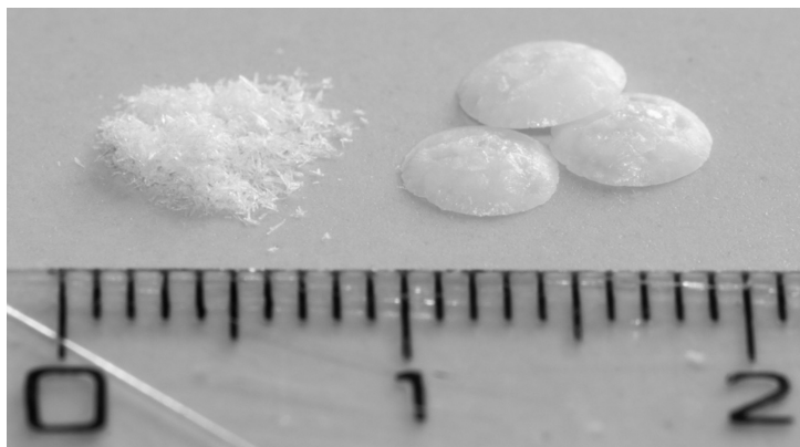
Figure 1. Shape and size of crystalline ETN (left) and melt-cast ETN pellets (right). The fine-scale divisions are in millimeters
